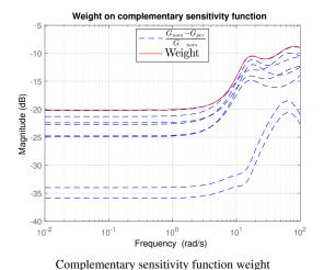
Fig. 11: Weights on sensitivity functions for regulator synthesis.
