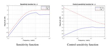
Fig. 9: Sensitivity and control sensitivity functions from regulator synthesis.
