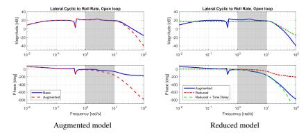
Fig. 7: Bode Plot for flight dynamics reduced models on roll axis.
