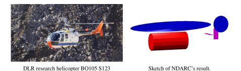
Fig. 3: Comparison between the actual BO105 and the helicopter resulting from NDARC's conceptual design.
