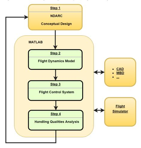
Fig. 1: Rotorcraft conceptual design tool architecture.
